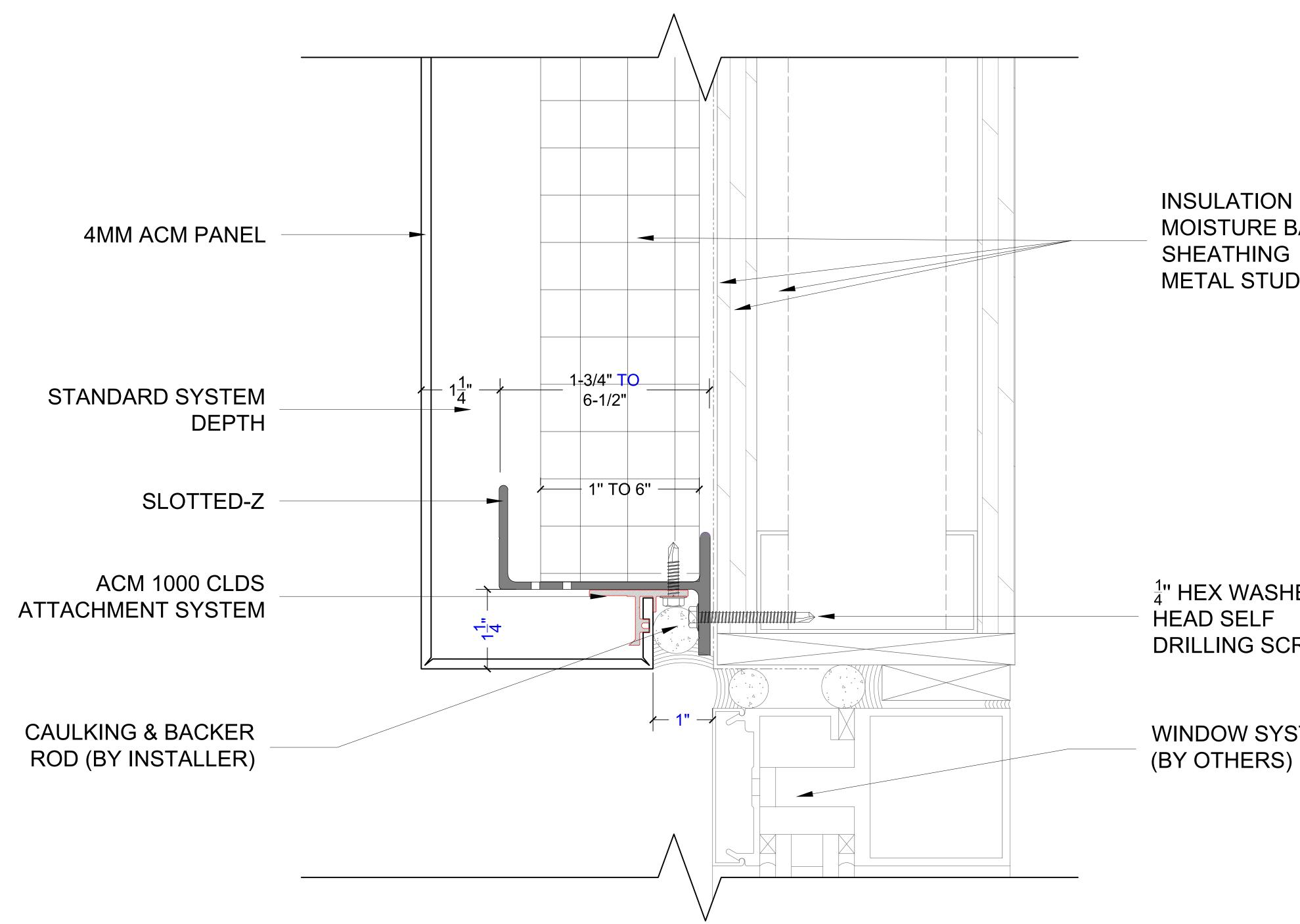
Clip-Lock Dry Seal Attachment System Header Detail
