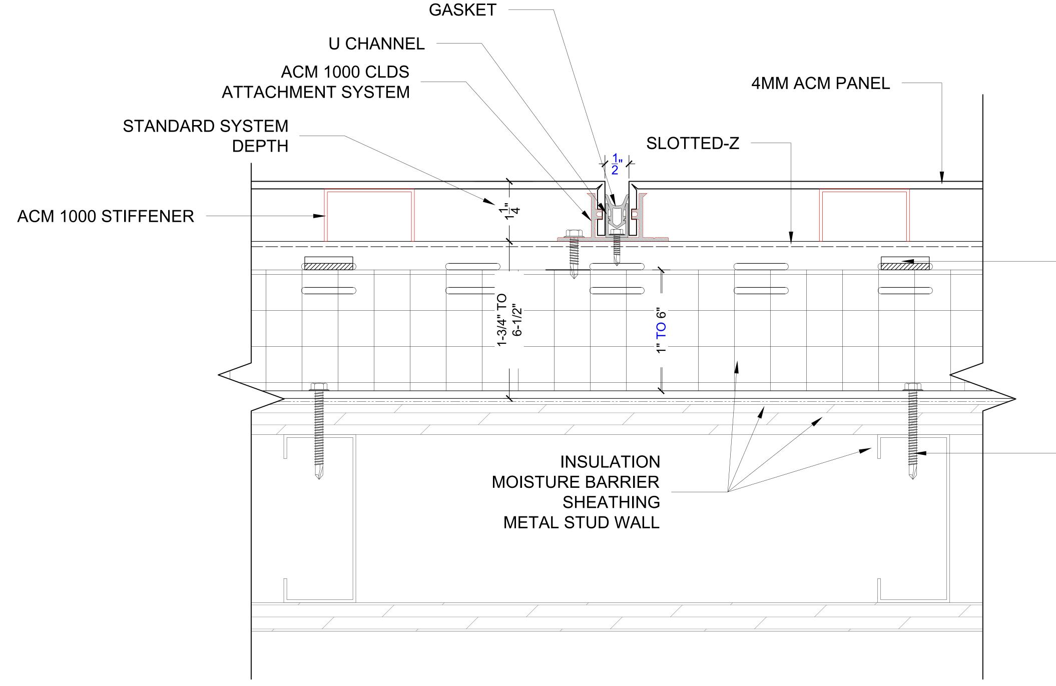
Clip-Lock Dry Seal Attachment System Vertical Joint Detail
