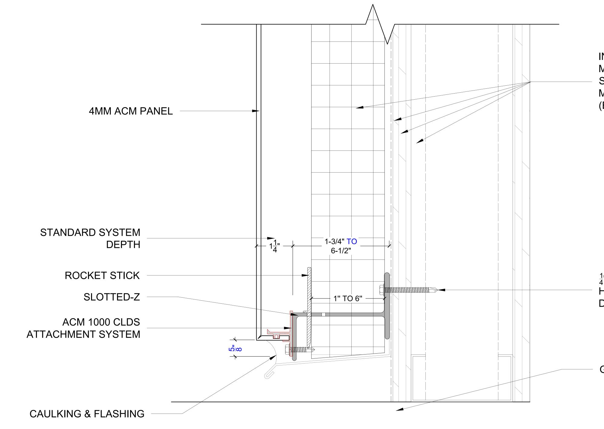
Clip-Lock Dry Seal Attachment System **Termination At Grade Detail**
