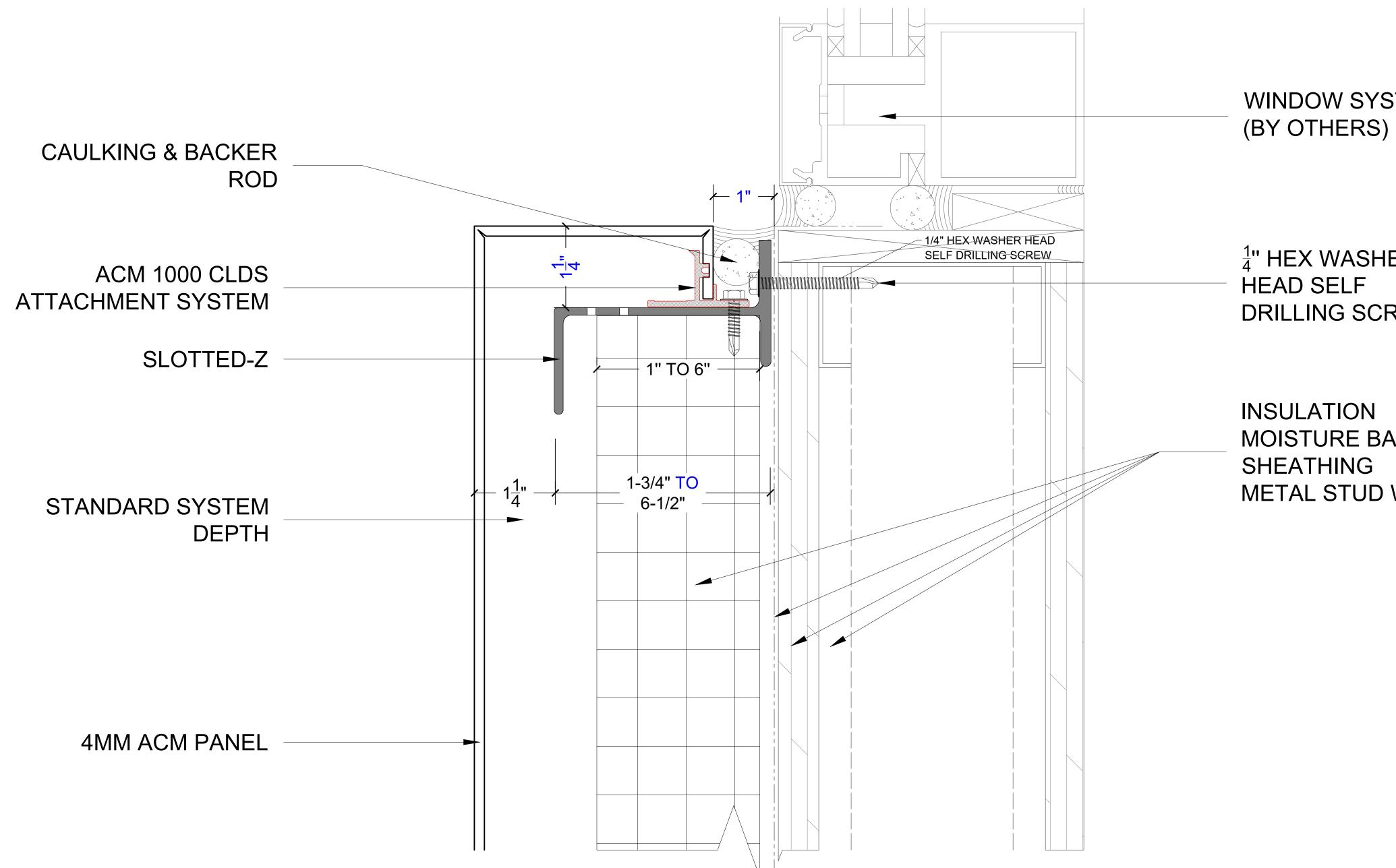
Clip-Lock Dry Seal Attachment System Window Sill Detail
