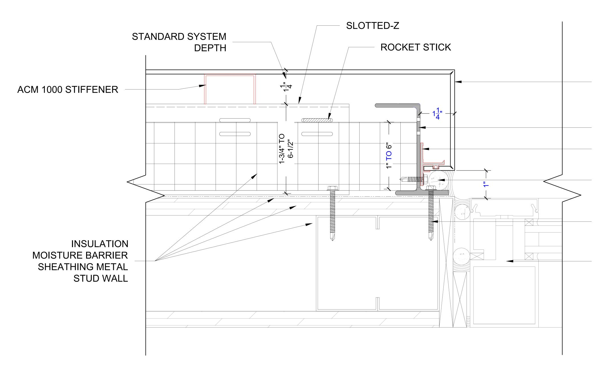
Clip-Lock Dry Seal Attachment System Jamb Detail
