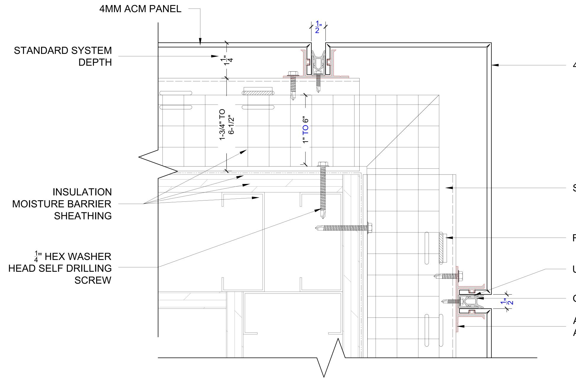
Clip-Lock Dry Seal Attachment System **Outside Corner Detail**
