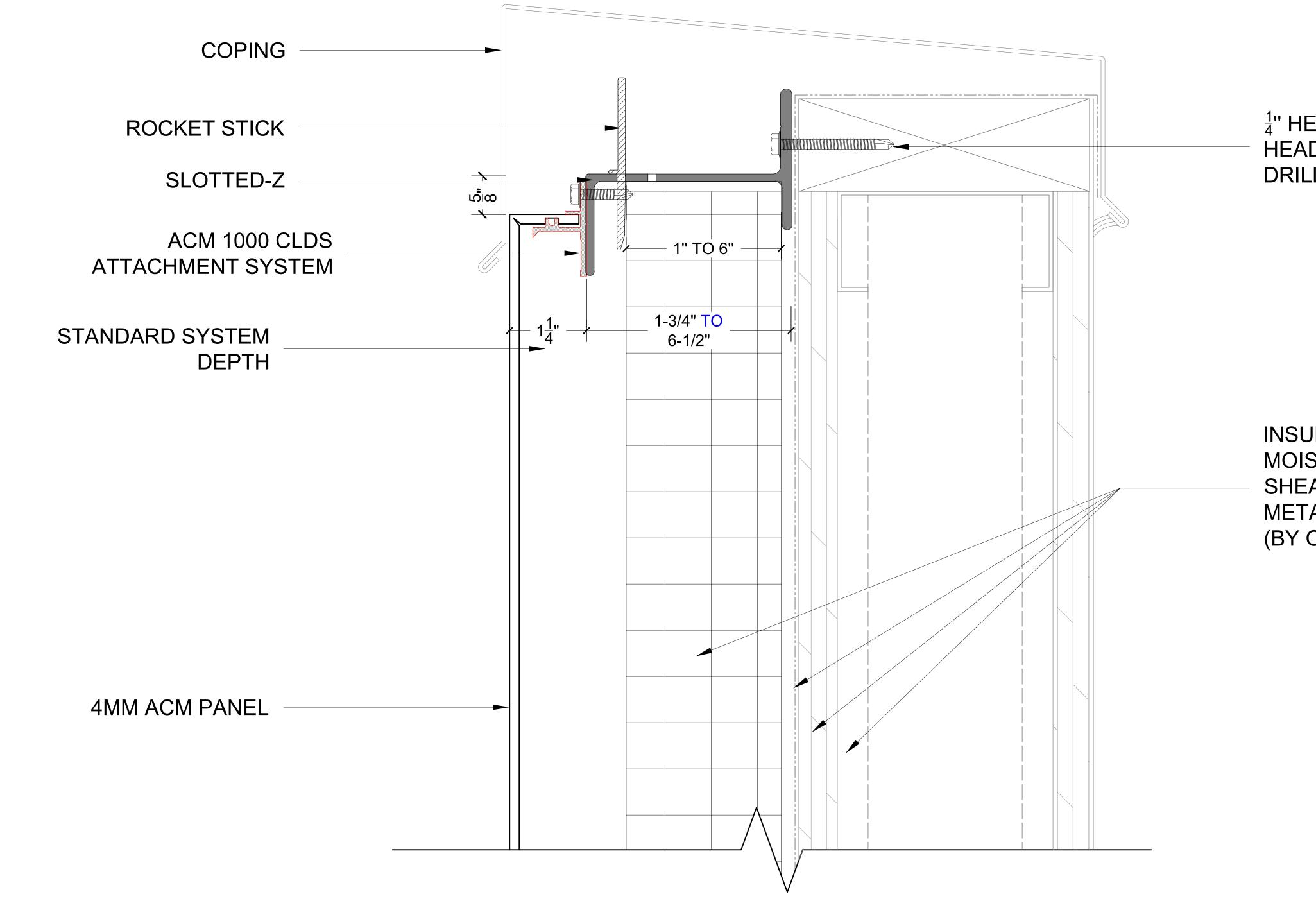
Clip-Lock Dry Seal Attachment System **Coping Detail**
