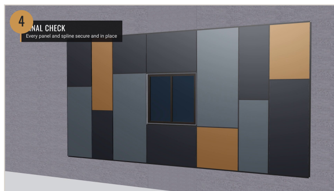
Final check: every panel and spline secure and fully in place.
